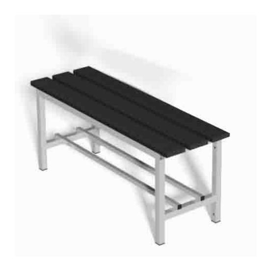
Changing room bench with seat only, 1 meter long, painted aluminum structure section 30x30 mm. Equipped with shoe shelf, seat with three black HPL slats, non-slip support points, closing caps on the tube ends. Dimensions = cm. 100x35x45h. The bench is supplied disassembled and complete with assembly kit.
