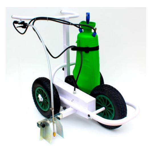
Spray field marker trolley for non-toxic liquid paints to be diluted with water, for lawns, consisting of: shell in tubular steel painted with polyester powders, blue white color, this product is lead-free and reflects the current environmental anti-pollution legislation; equipped with three pneumatic wheels diameter mm.350, polyethylene pressure bottle capacity Lt. 14, equipped with safety valve, the components of the bottle comply with directives 97/23 / EC Weight of the empty trolley Kg. 24
