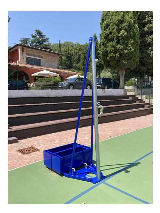
**Steel trellis system** composed of 2 painted steel case holder frames complete with 2 8mm thick plates. resting on the ground and 4 boxes in painted steel of the size of 90cm. per side 30x30cm. Central upright in round tube diam. D = 70mm and thickness 3mm,
