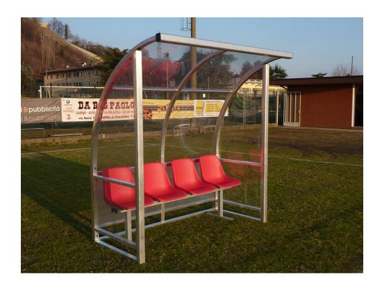
Bench model "Strong" 1 meter (2 places), covers and sides made entirely of aluminum with 60x70 mm oversized front safety uprights. Semi-transparent honeycomb polycarbonate cover 4 mm thick. Seat frame in hot galvanized steel and polypropylene shells with back.
