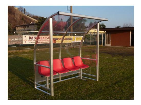
Bench model "Strong" 5 meters (10 seats), covers and sides made entirely of aluminum with 60x70 mm oversized front safety uprights. Compact transparent polycarbonate cover 3 mm thick. Seat frame in hot galvanized steel and polypropylene shells with back.
