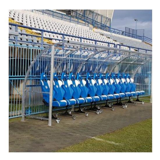
Team shelter model "Strong Plus" 4 m. long (8 seats), in aluminium, front struts construction mm. 60x70, policarbonate panels transparent thickness mm. 3, seats in polypropylene.
