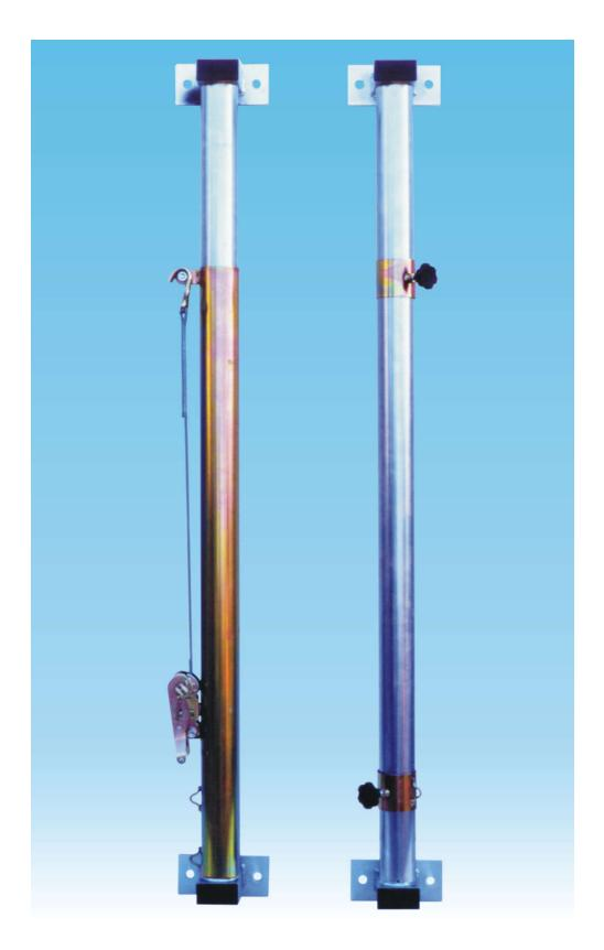
Wall-mounted volleyball system with net tensioner, in galvanized steel tubing diam. 70 mm, length 1500 mm, to be fixed to the wall with plates using plugs. Adjustment of the net by means of sliders with telescopic sliding and tensioning winch equipped with belt for hooking the net.
