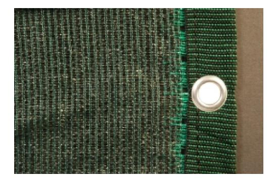
Windbreak-sunscreen tarpaulin available in various weights, rashel machine weaving with polyethylene flat yarn. 100% high density, stabilized against ultraviolet rays, with eyelets every 50 cm.
