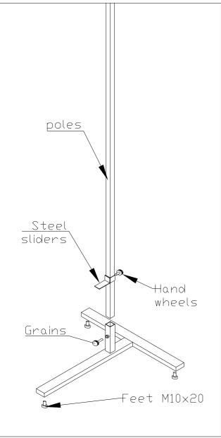
Light alloy vertical poles, heavy "t" basement height mt. 2.5, in varnished steel. Aluminium pole mm30x30 and steel slider.
