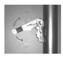
To net tension, pull the band using the winch, moving up and down the knob as the image show.
