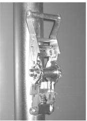
To increase and decrease band tension, hold the winch blade down and move the lever up as pictured, then grasp the band and pull to remove it.
