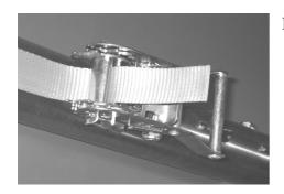
Insert the band into the gear.
