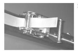
Insert the tape inside the winch.
