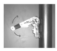
To tension the net, pull the tape with the use of the special winch by moving the knob repeatedly first upwards and then downwards as in the image alongside.
