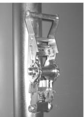
To remove or decrease the tension of the belt, hold down the blade of the winch down and move the lever upwards as in the drawing. Then grab the ribbon and pull to remove it.
